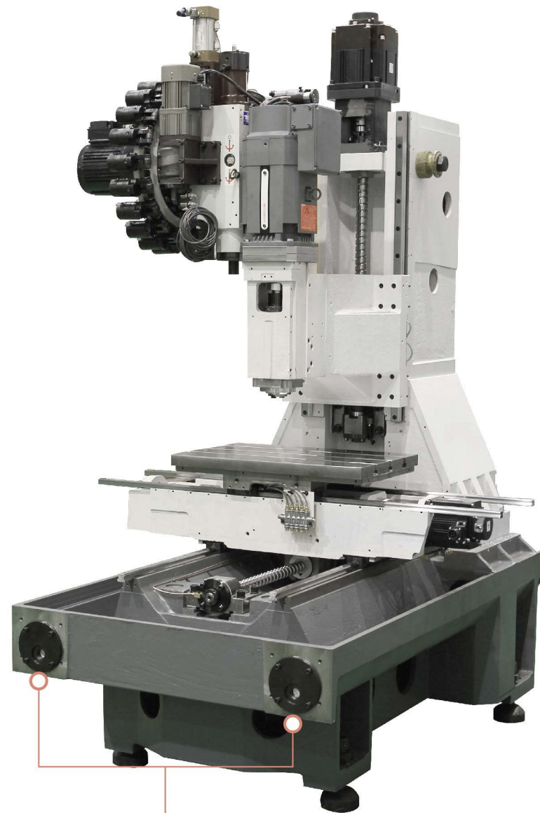
Dual-chip disposal design:TMV-510AII/CII
