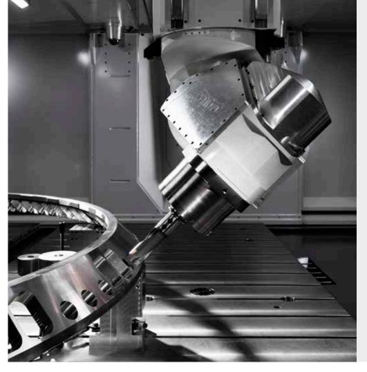
Machining of slewing bearing
